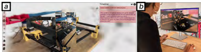
Figure 4: (a) The local user’s video is placed as a floating screen in the SplatOverflow scene and aligned to the same perspective it was filmed in. (b) The remote maintainer reviews the local user’s issue by inspecting the vacuum nozzle in the splat and CAD model.
